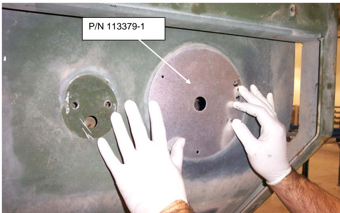
Figure 26. Install the Headlight Covers.
