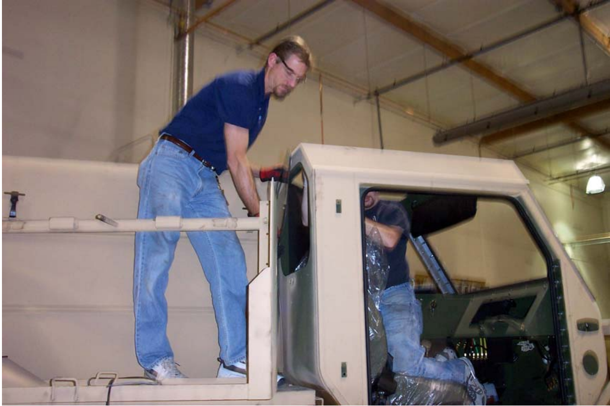
Figure 13. Remove the Rear Cab Window.
