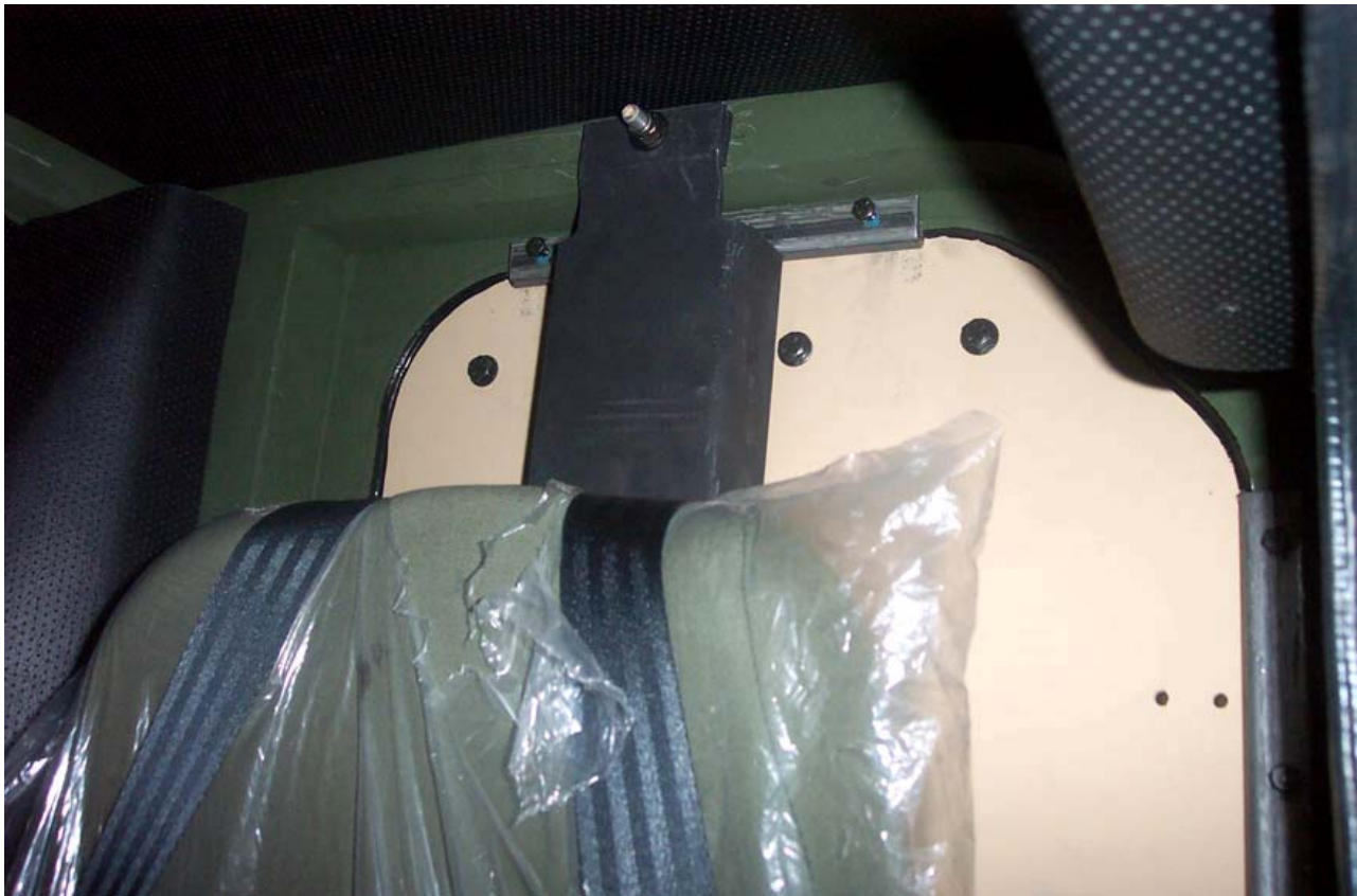
Figure 29. Move the Harness Bracket to the inside for increased clearance for the Rear Cab Armor Panel Bracket.
