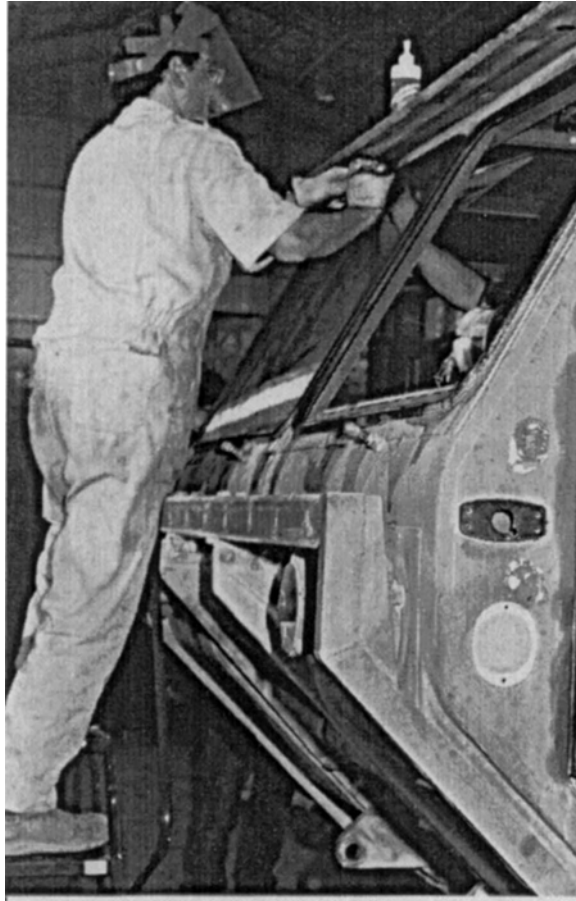
Figure 12. Remove the windshield half.
