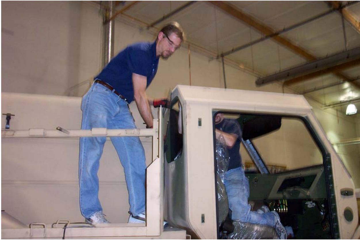
Figure 13. Remove the Rear Cab Window.
