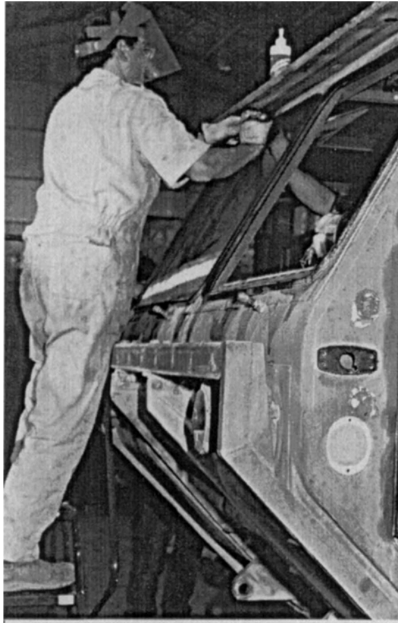
Figure 12. Remove the windshield half.
