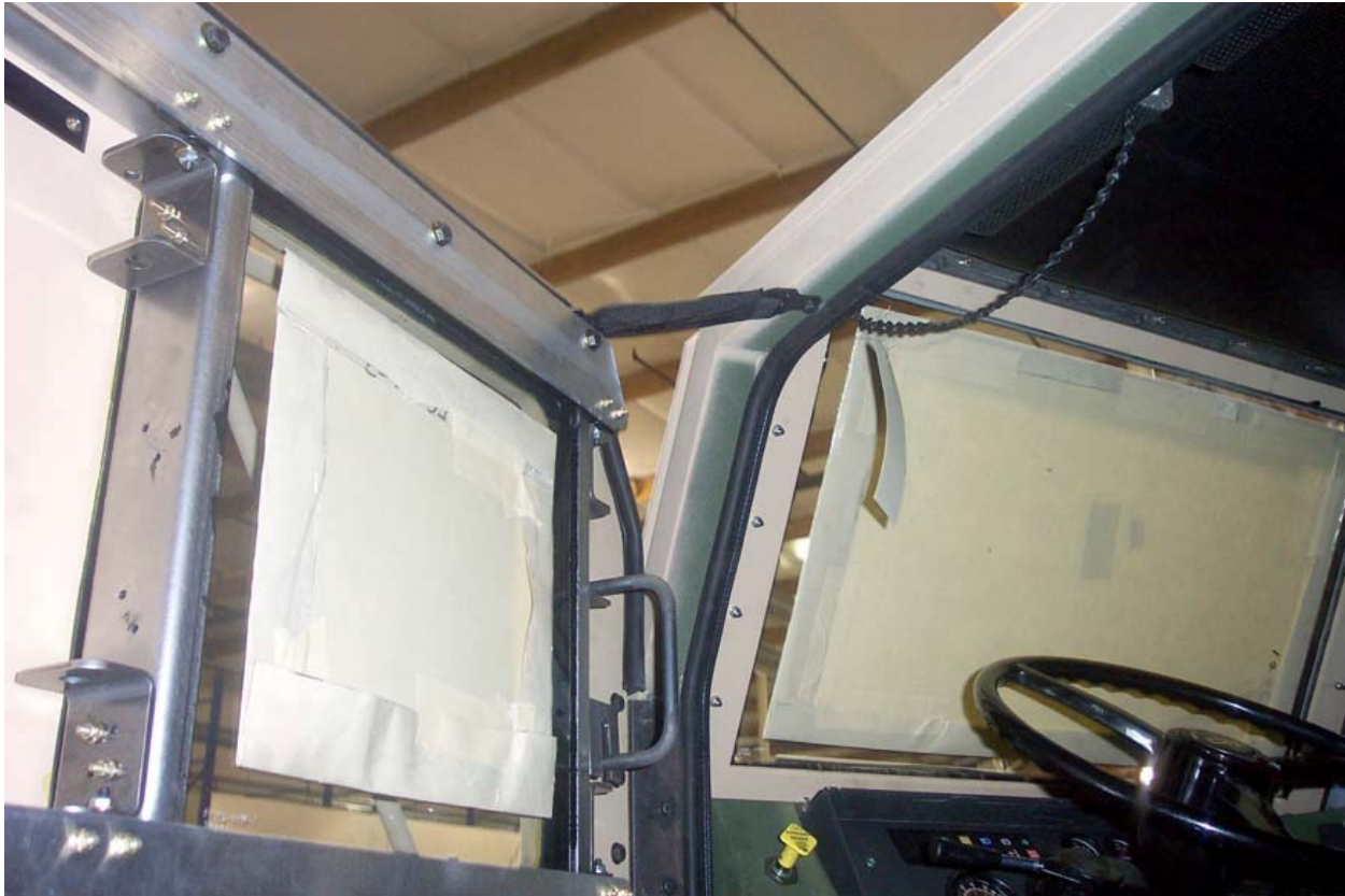
Figure 34. Install the new Attachment Strap to the Armored Door Assembly.
