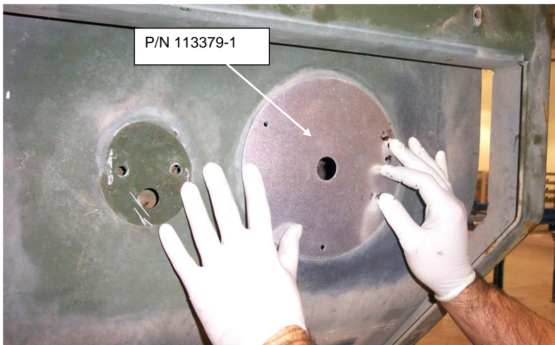
Figure 23. Install the Headlight Covers.
