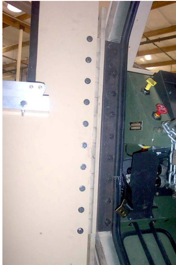
Figure 32. Install the Armored Door Assembly to the cab (driver's-side door shown).
