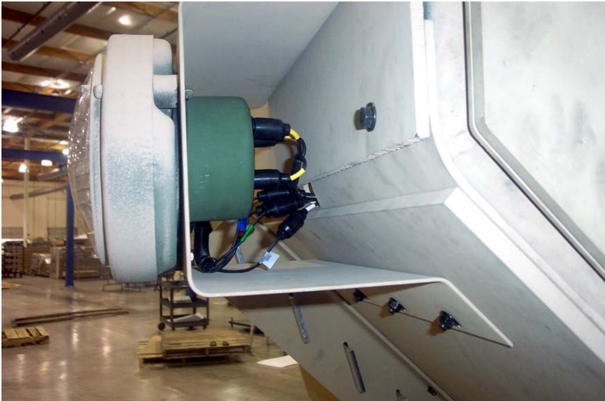
Figure 28. Left-hand Headlight Bracket Installed.
