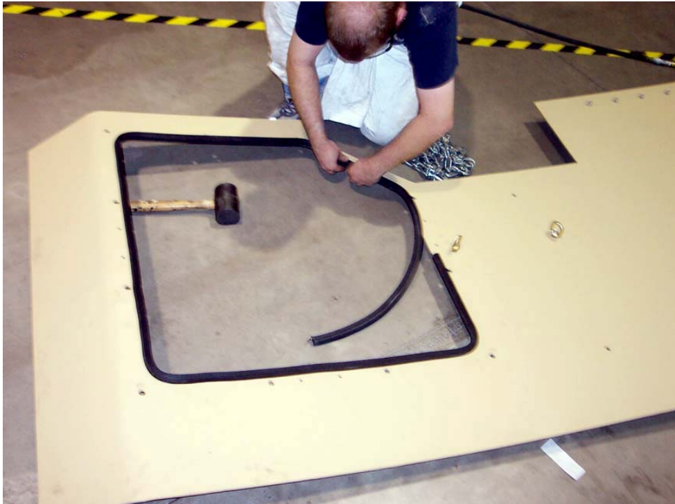
Figure 40. Install the hatch seal.
