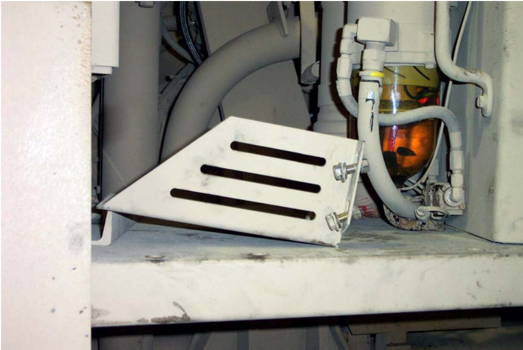
Figure 9. Remove the Fuel-Air Separator Guard.
