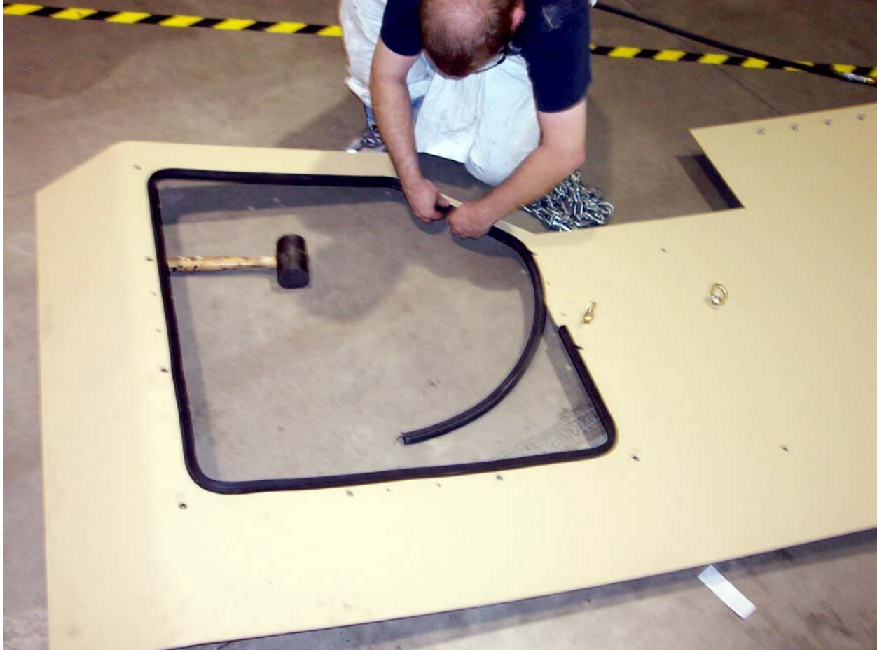
Figure 45. Install the hatch seal.
