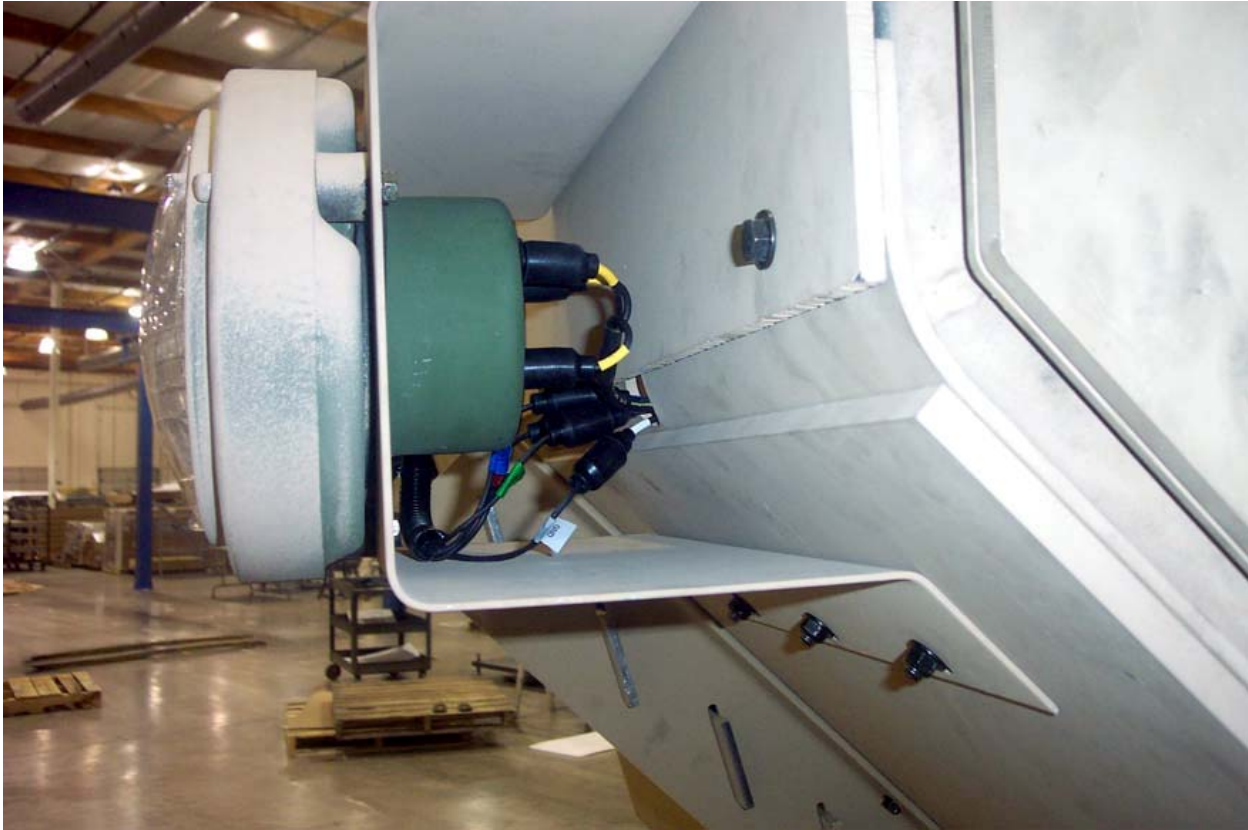
Figure 25. Left-hand Headlight Bracket Installed.
